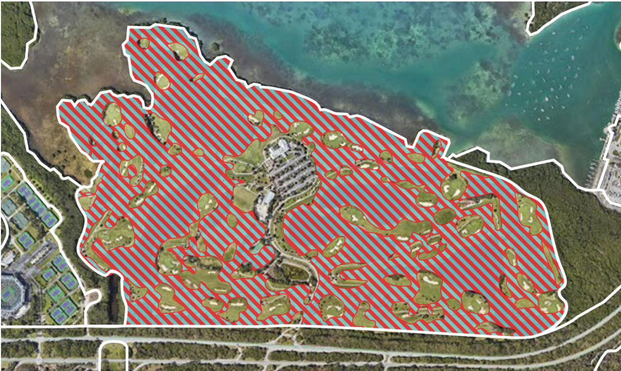
A majority of the Golf Course area is at 4ft above sea-level or lower, making it vulnerable to sea level rise and storm surges.
