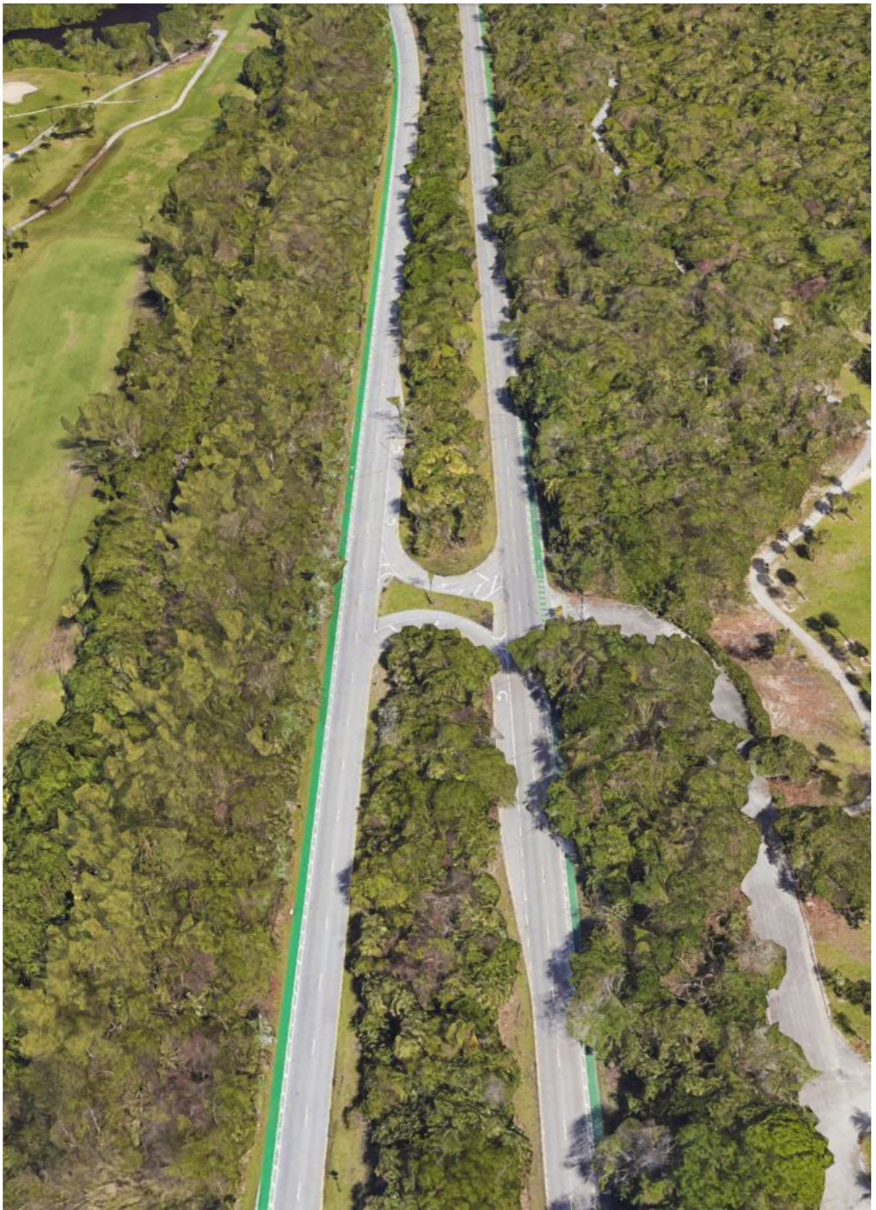
Four lane Crandon Boulevard with around turns and poor visibility due to dense vegetation
