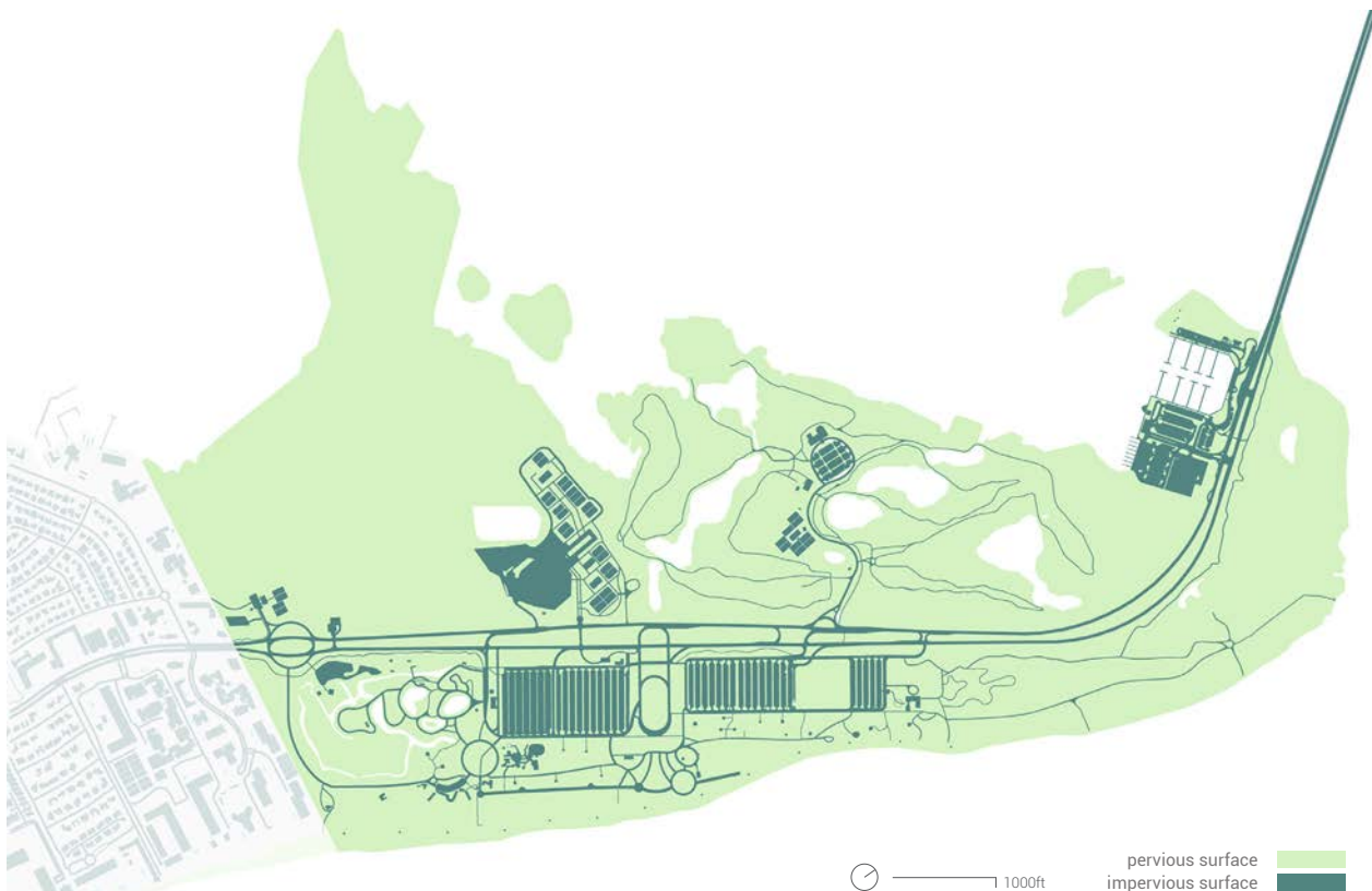
Impervious surface 10% of total park area
